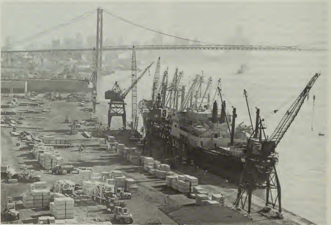
An older breakbulk cargo vessel carries her own cranes onboard for loading and off-loading cargo on pallets. This would allow off-loading of military cargos in undeveloped or battle-damaged port areas, but loading and unloading of this type of vessel are labor-intensive and time-consuming.
